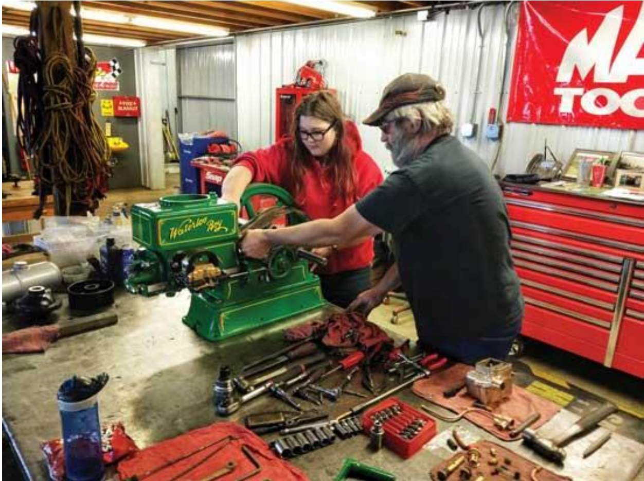
Emma and Mike trial fit the crank guard that had to be made for the Waterloo Boy. They're usually missing or in poor condition.
