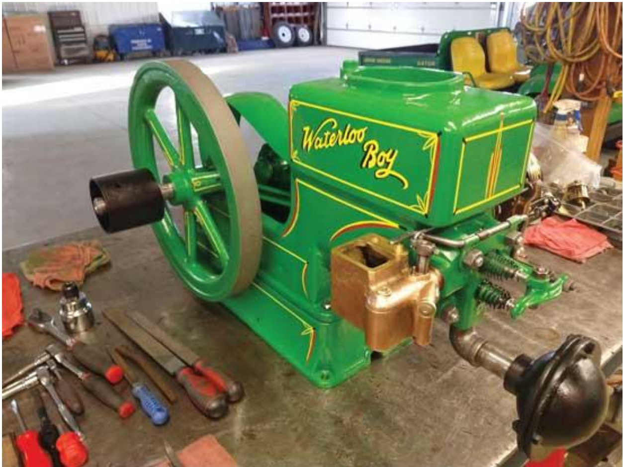
The finished crank guard in place, work turned to finish assembling the mixer.
