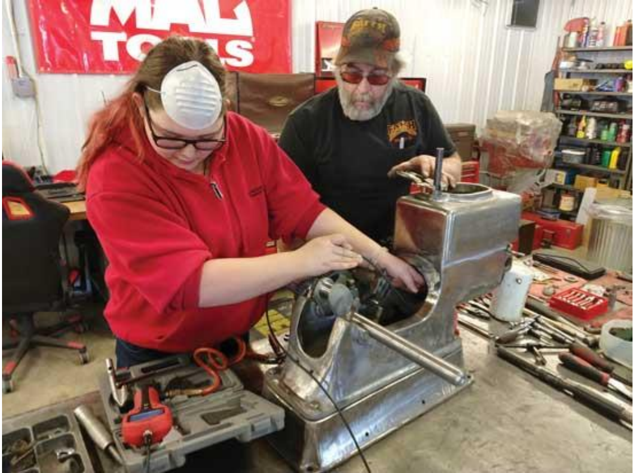
Emma checks the engine's cylinder bore using a digital micrometer as Mike looks on.
