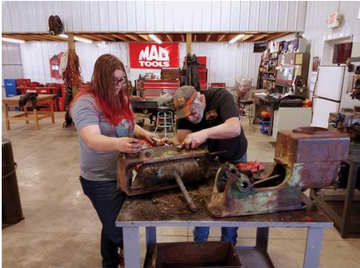
Emma and volunteer Mike Albright work on stripping the Waterloo Boy's engine base. Here they're shown coaxing the gas tank from the base.
