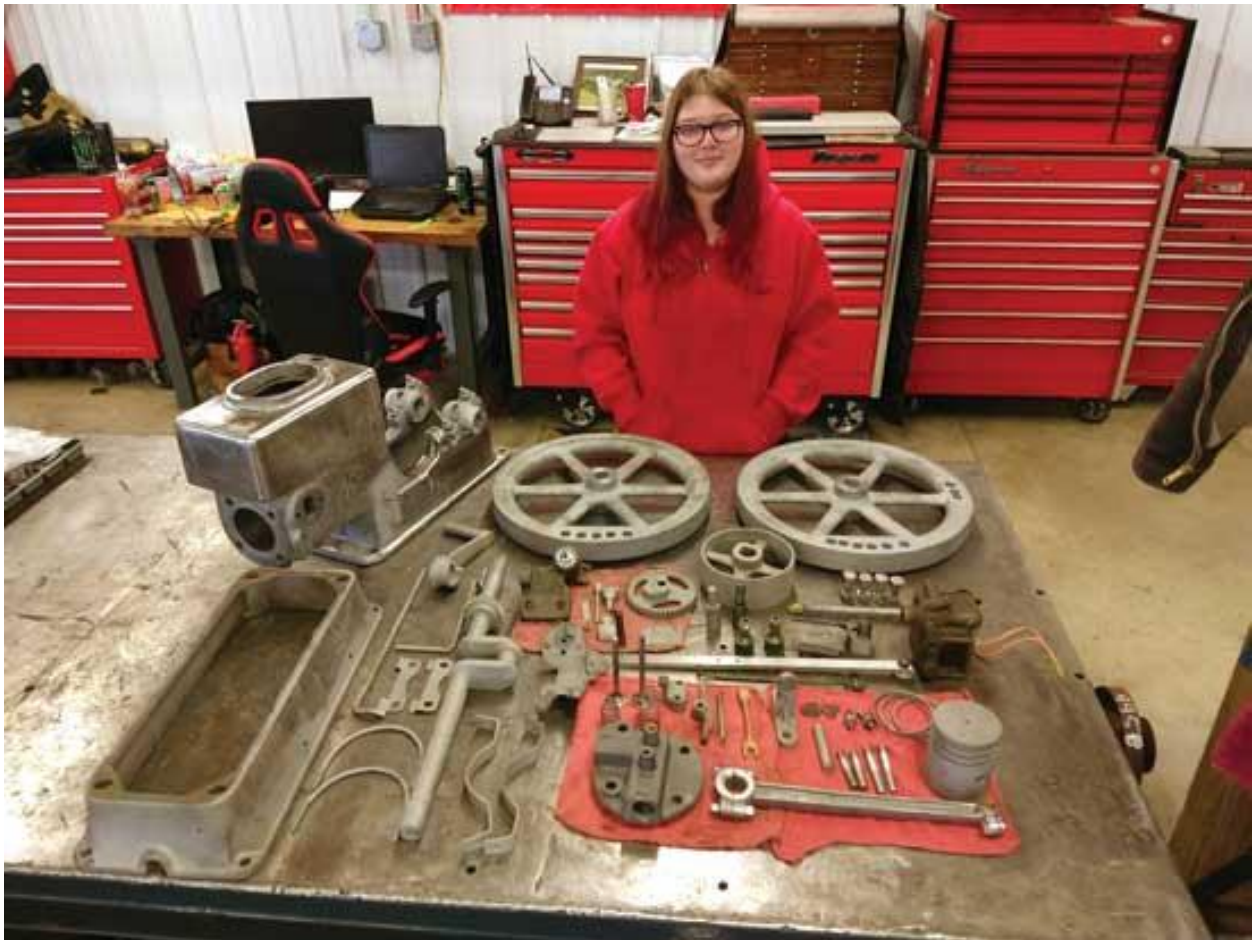
Emma with the Waterloo Boy, stripped, cleaned and ready for reassembly.
